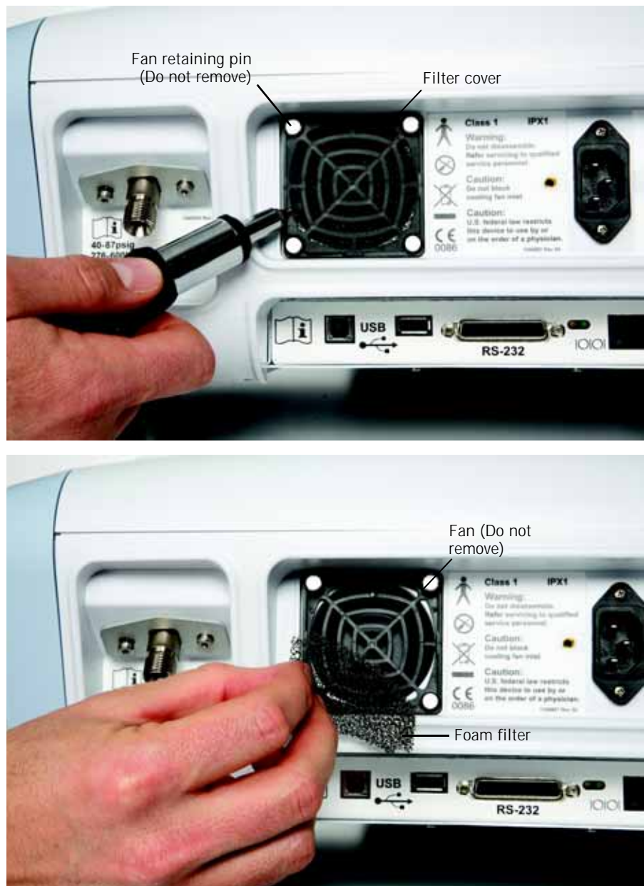
Figure 9-2: Replacing the cooling fan filter
