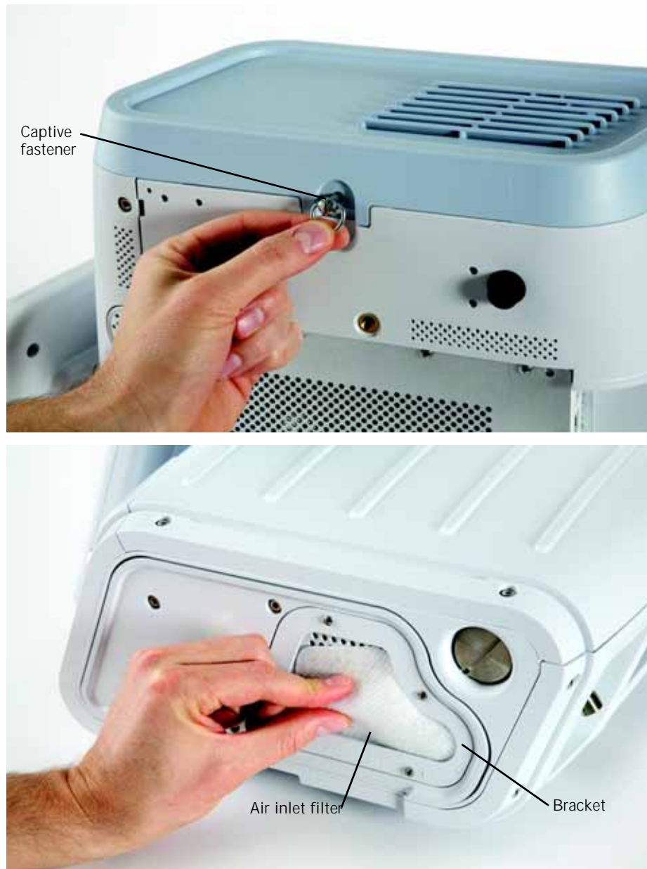
Figure 9-1: Replacing the air inlet filter
