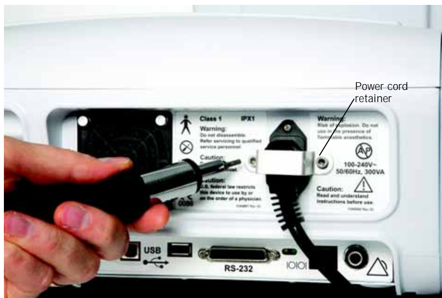
Figure A-4: Installing the power cord retainer
