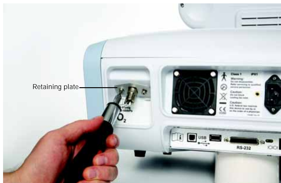
Figure A-3: Installing the oxygen inlet connector
