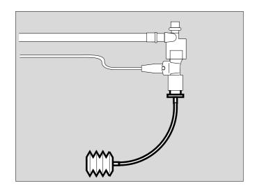
When an extractive monitor is used, a vacuum may be generated in the airway if the inspiration hose becomes blocked.
