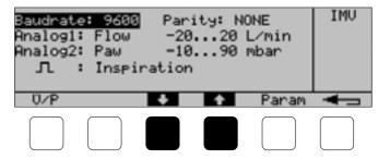
Operation Configuring RS 232 interface Setting the printer
