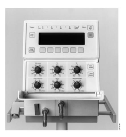
The front panel consists of the **control panel** and the **display panel** with a screen.
