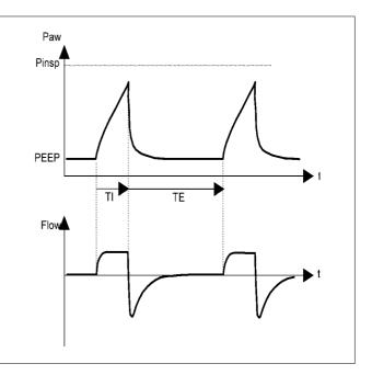
Operation Selecting the Ventilation Mode and Additional Functions IPPV / IMV
