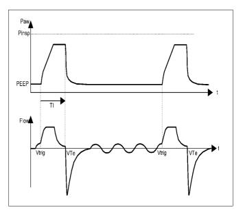
In the case of a serious leak in the tube, the expired VT may (just as in other ventilation modes) be greater than that measured at the expiration connector. The inspiratory tidal volume will then differ from the expiratory tidal volume. If, in the course of a ventilation stroke, the actual inspiratory VT exceeds the VTe of the previous stroke by an amount which depends on the actual leakage, the Babylog 8000 plus terminates the inspiration stroke.
