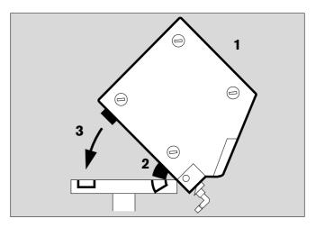
• Place the shelf on the Babylog 8000 plus, engaging the two tabs in the slots at the rear of the unit.
