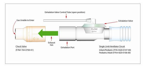
CHECK VALVE CONNECTION TO BREATHING CIRCUIT: FIGURE 12
