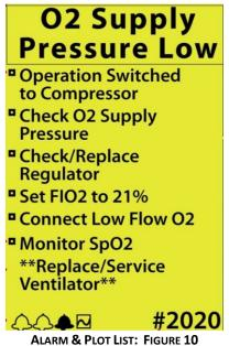
Figure 10 is an illustration of what is seen if there are several alarms. The Alarm message refers to the alarm bell that is dark. The Operator can cycle through the various alarms by turning the encoder dial. If there are less than 5 alarms, this alarm list will also include a "plot" icon, where the alarm screen will be replaced by the Pleth and Pressure/Time plots.
