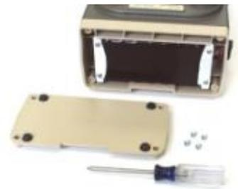
The EMV+ Battery Pack is wired to a mating plug-and-socket connector that remains electrically-attached to the EMV+.
