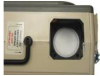
Set the lower segment of the Compressor Inlet Fitting Assembly into the EMV+ making sure that its alignment pin mates.
