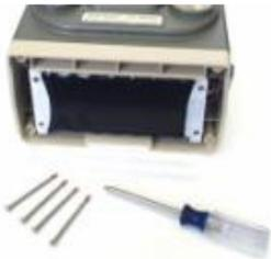
Remove the four (4) 6-32 x 2 ¼ Phillips Pan Head screws that hold the Battery Pack and its integral mounting bracket to the EMV+ Lower Case.
