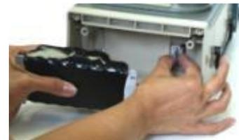
**WARNING!** Make sure that none of the Battery Pack wires get pinched between the bracket and case enclosure.
