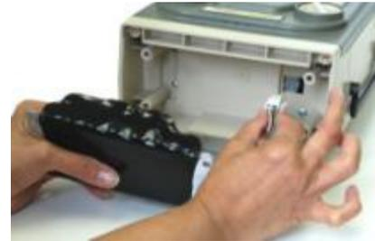
Replace the old Battery Pack with one that is new.
