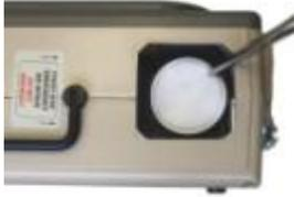
Remove the Disk Filter using the hemostat or tweezers and replace it with a new, clean filter. Make sure that the filter sits flat on the shoulder in its recessed area.
