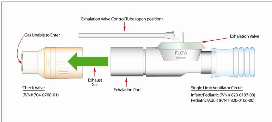
CHECK VALVE CONNECTION TO BREATHING CIRCUIT: FIGURE 12
