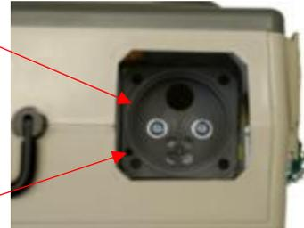
Set the upper segment of the Compressor Inlet Fitting Assembly into the lower segment making sure that its alignment pin mates.
