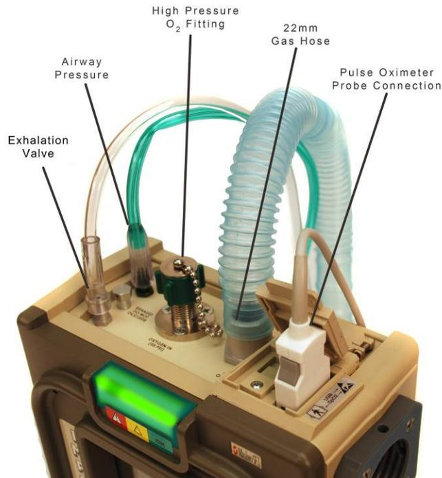
VENTILATOR CIRCUIT, DEVICE CONNECTIONS: FIGURE 5
